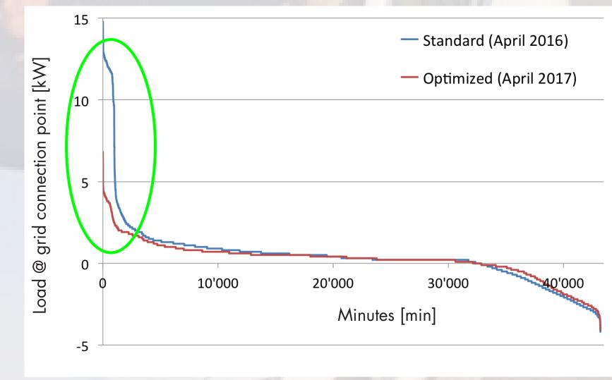
Active load management of heat pump and EV charge for PV optimization not only increases PV self-consumption but reduces strain on the power grid. Especially the high demand peaks of fast EV charge are almost eliminated.
