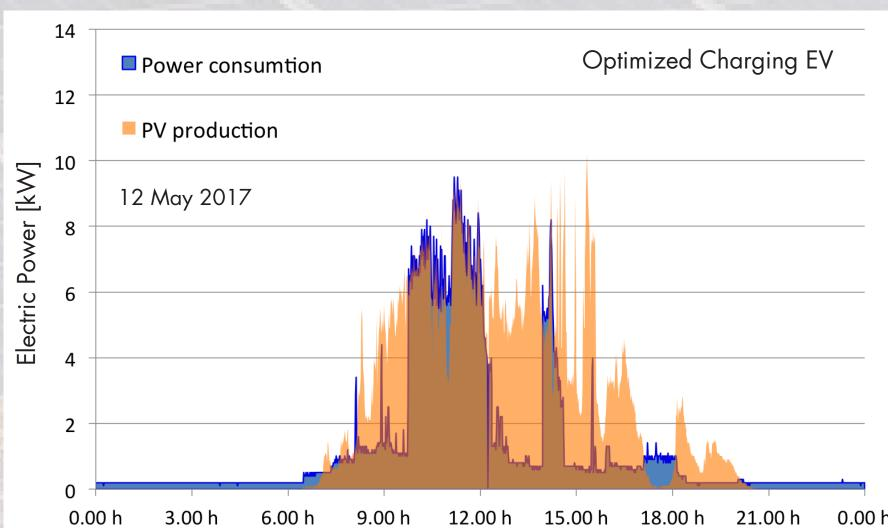
Under EV standard charge much energy is drawn from the grid even on a sunny day. Most PV energy is fed into the grid. Under PV optimized charge PV production is absorbed precisely by the car battery. Hardly any energy is drawn from the grid.
