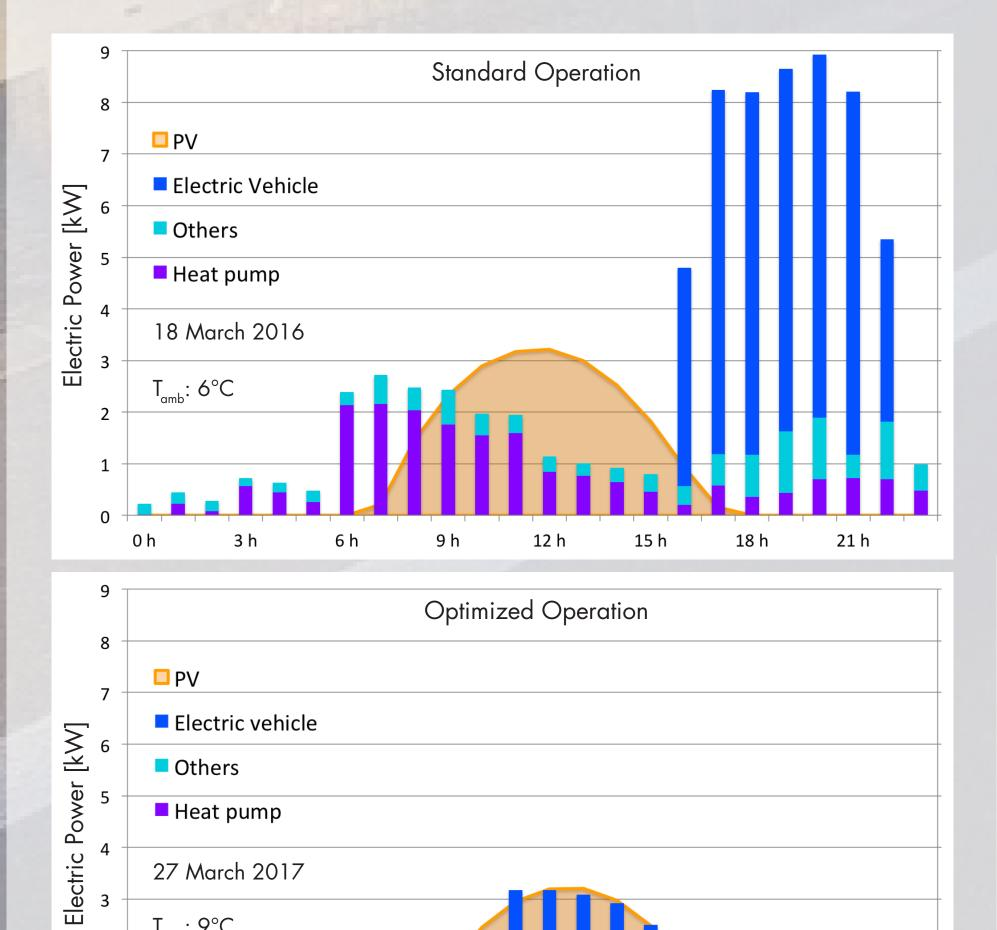
With manufacturers standard settings the heat pump doesn't use PV production optimally. Actively controlling both, EV charge and heat pump operation, PV production is used optimally within the house and less energy is drawn from the grid.
