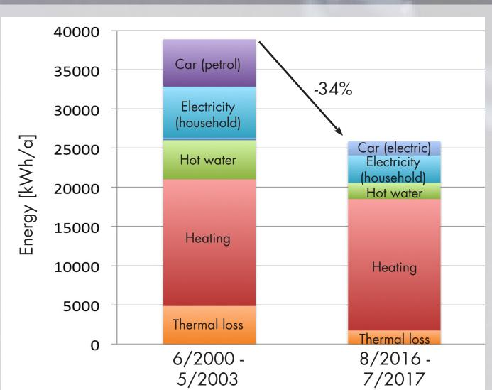
Energy consumption is reduced by 34% realizing various efficiency measures: Reducing thermal losses and standby consumption, exchanging inefficient appliances, increased efficiency with EV.
