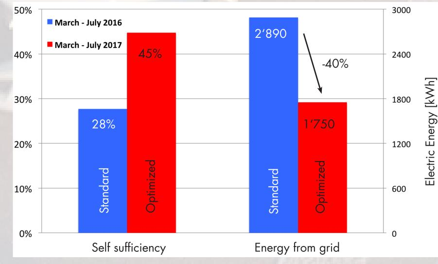
PV optimized operation of heat-pump and EV charge increases degree of self-sufficieny from 28 % to 45 % and reduces the amount of energy drawn from the grid by 40 % in the comparative period.
